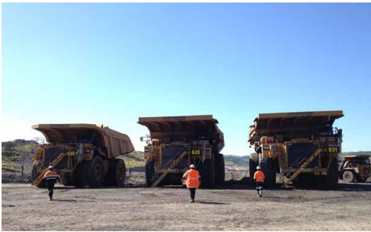
The main overburden fleet includes Komatsu PC4000s and Caterpillar 789C dump trucks.
